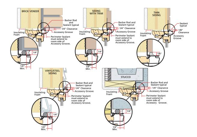
A. **Insert backer rod** into the space around the window to provide approximately 1/4" clearance between the backer rod and the exterior face of the exterior finish material.
